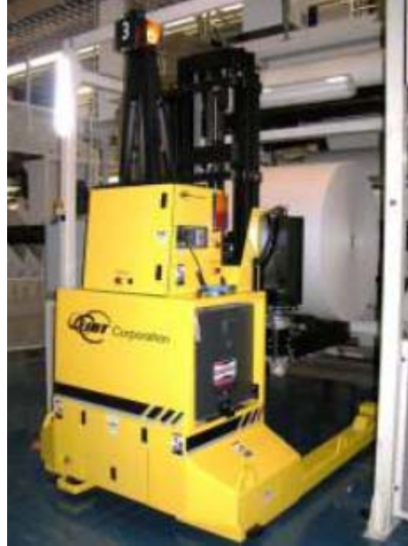
AGVs deliver prepped roll to lay down racking in a printing center warehouse
