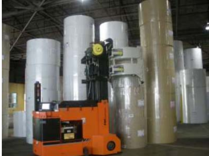
3 Roll Clamp vehicles stack rolls and 3 Counterbalanced Fork vehicles stack pallets
