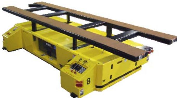
*Low profile design allows SGV to drive under conveyor stands to pickup and deliver refrigerators*
