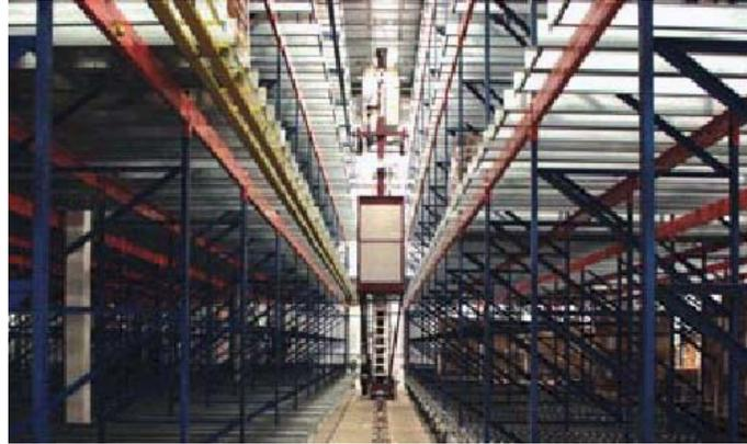
*"At only 33' high, the facility's height is typical of conventional warehouses. But with our High Density AS/RS technology, its dense 4 level cubic storage requires a smaller building footprint, thereby having less impact on the environment around the facility."*
