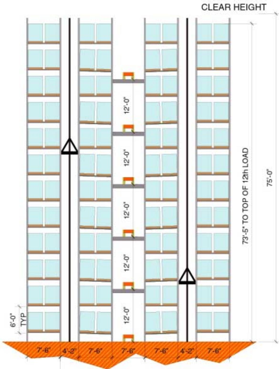
FIGURE 5 - ELEVATION VIEW: AS/RS CONCEPT
