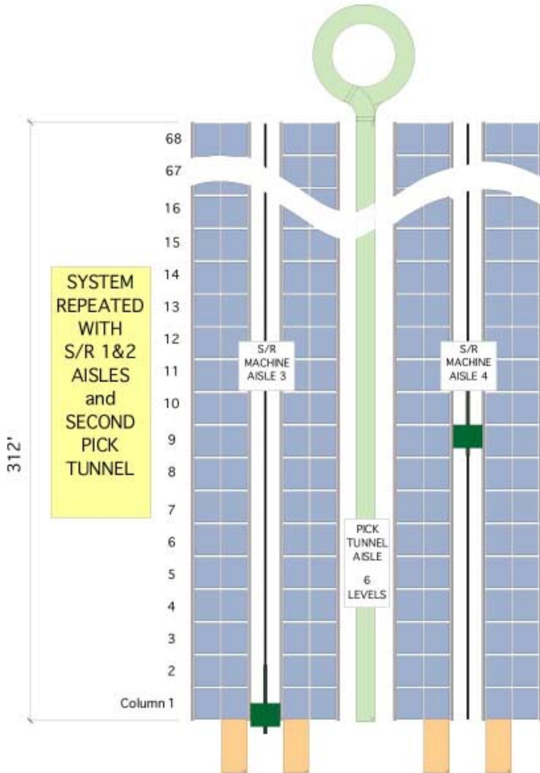
FIGURE 4 - PARTIAL PLAN VIEW: AS/RS CONCEPT
