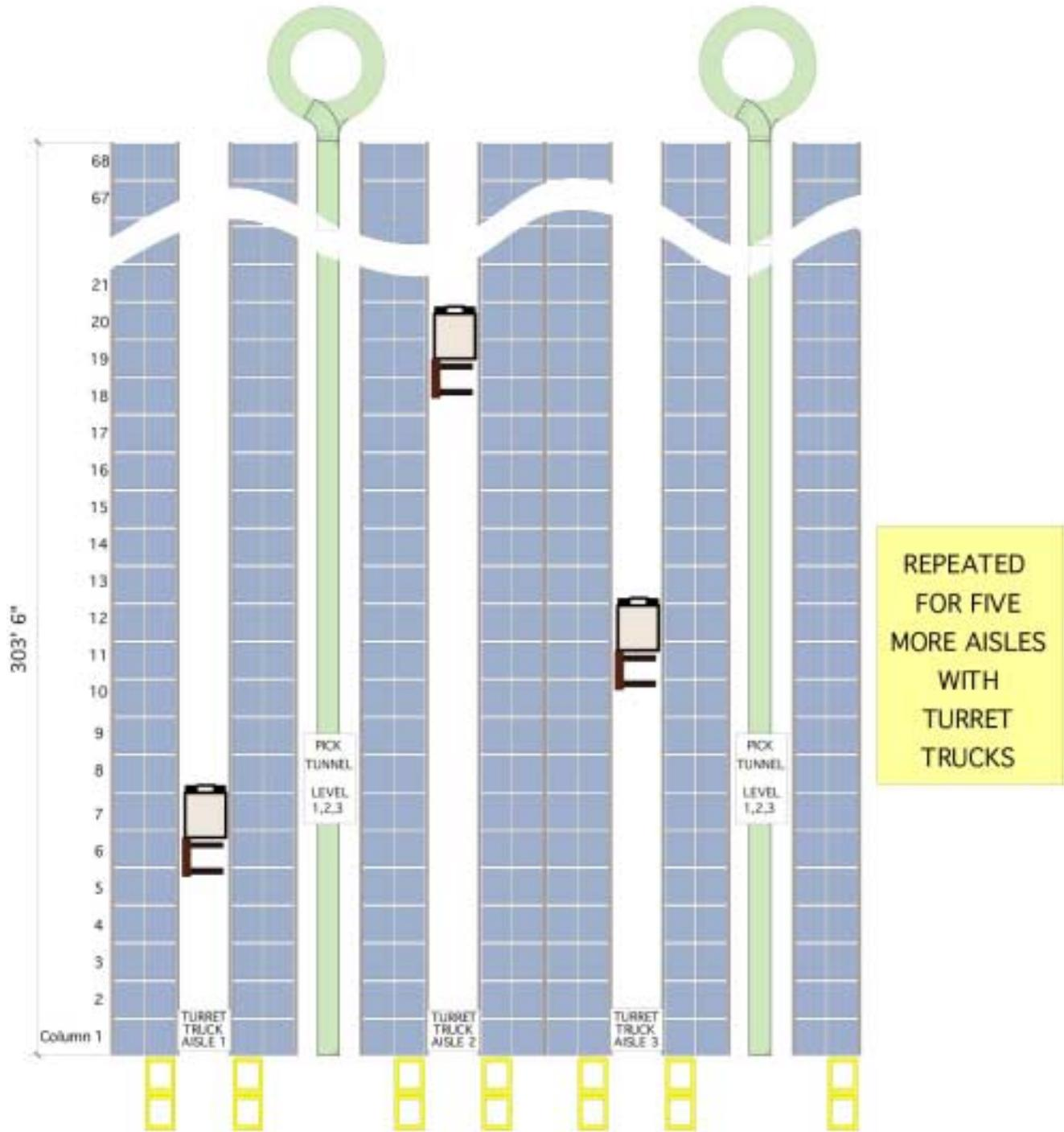
FIGURE 1 - PARTIAL PLAN VIEW: VNA CONCEPT
