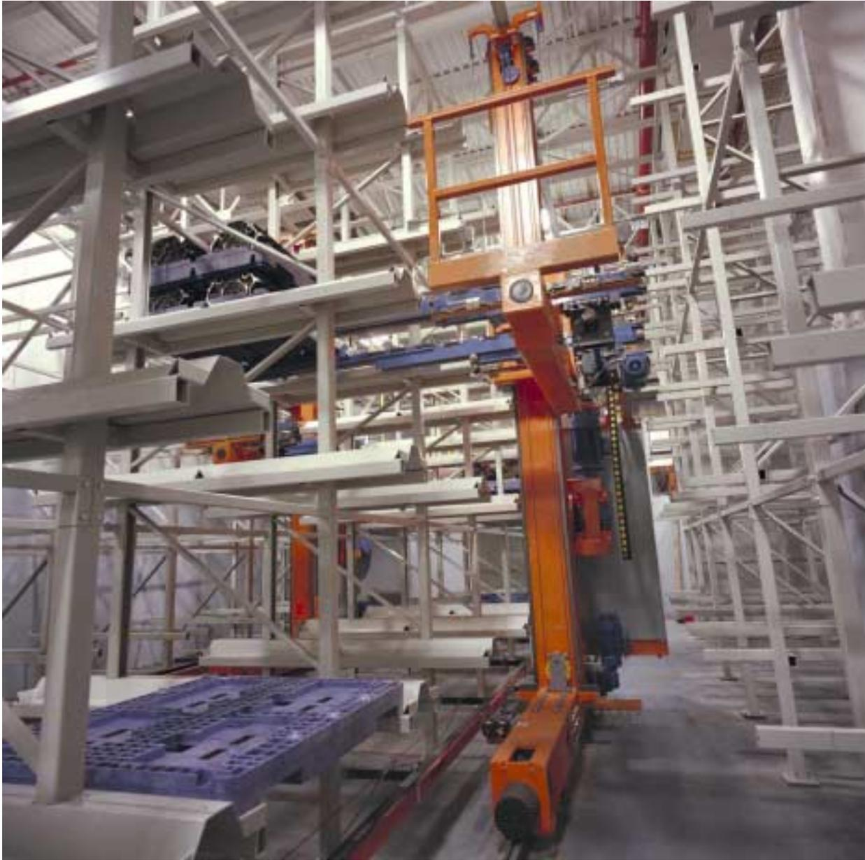
**Figure 6b. –View of an Empty Pallet in the Rear Position and a Single Aisle Unit Load AS/RS with its Shuttle Forks Extended to a Double Deep Load**
