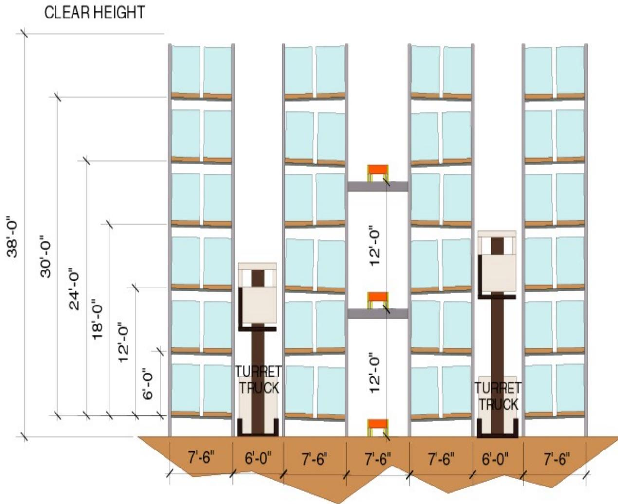
FIGURE 2 - ELEVATION VIEW: VNA CONCEPT
