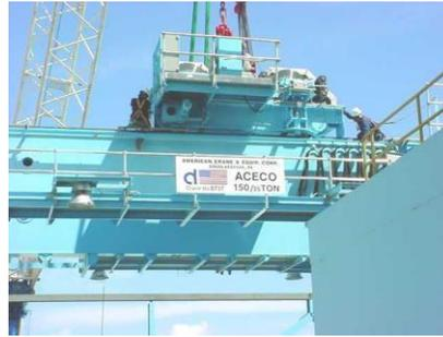
*150 Ton Single Failure Proof Cask Handling Crane*
