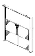
**10.2.5 Horizontal Sliding Type Gate Assembly.** This style gate operates in the same matter as a vertical rising gate
