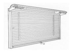
itself does not require a lot of space. Some disadvantages are that it is slow in operation, may require considerable maintenance, and it is mounted over the gate opening and may limit the load height. It may be of the manual or powered variety.
