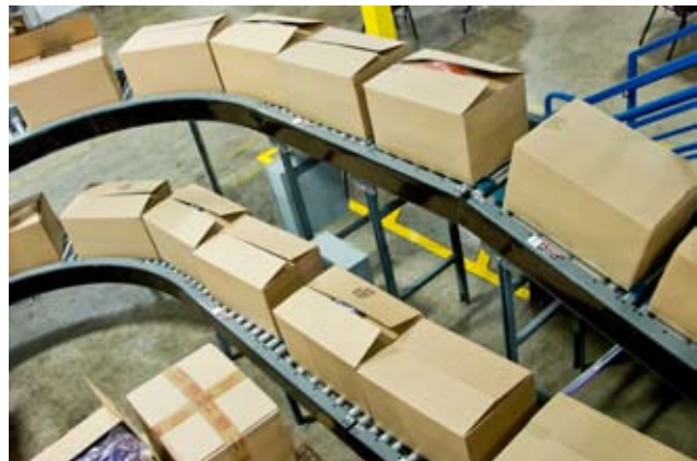
MDR accumulation buffer prior to sort transfer.
