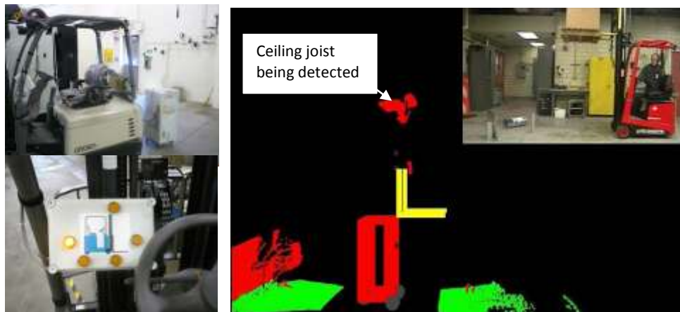
Figure 16 – (top-left) 3D LIDAR sensors mounted on a forklift and integrated with simple operator alerts. The obstacle is behind the forklift and (bottom-left) the alert indicates the location of the obstacle relative to the forklift, (right) high-lift obstacle detect sensor mounted on the forklift frame and raised (upper right inset photo is shown reversed from the data) to capture data of the ceiling joists.
