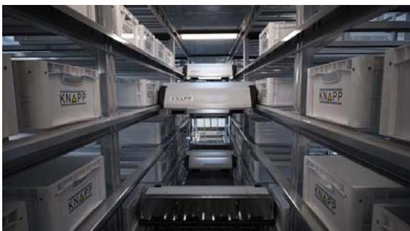
Figure 2: Shuttle system (OSR Shuttle by courtesy of KNAPP)
