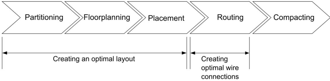
Figure 2: Basic process to create a microchip design
