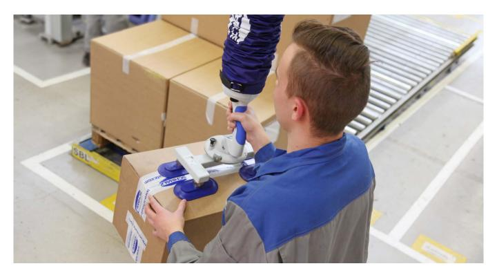
Ergonomic lifting aids are always in demand, especially in the logistics. One the one hand, the global trade is increasing steadily. On the other hand, the demographic change promotes the awareness of ergonomics and health protection at work. The new vacuum tube lifter Jumbo Flex 50 from Schmalz is the answer to these developments. The derivative of the successful tube lifter series offers many more benefits besides the increased lift capacity of 50 kg.
