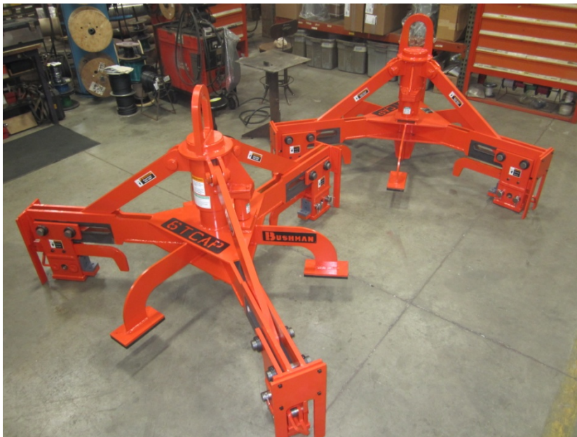
Custom engineered BUSHMAN® lifter picks up one of several sizes of welded frames.
