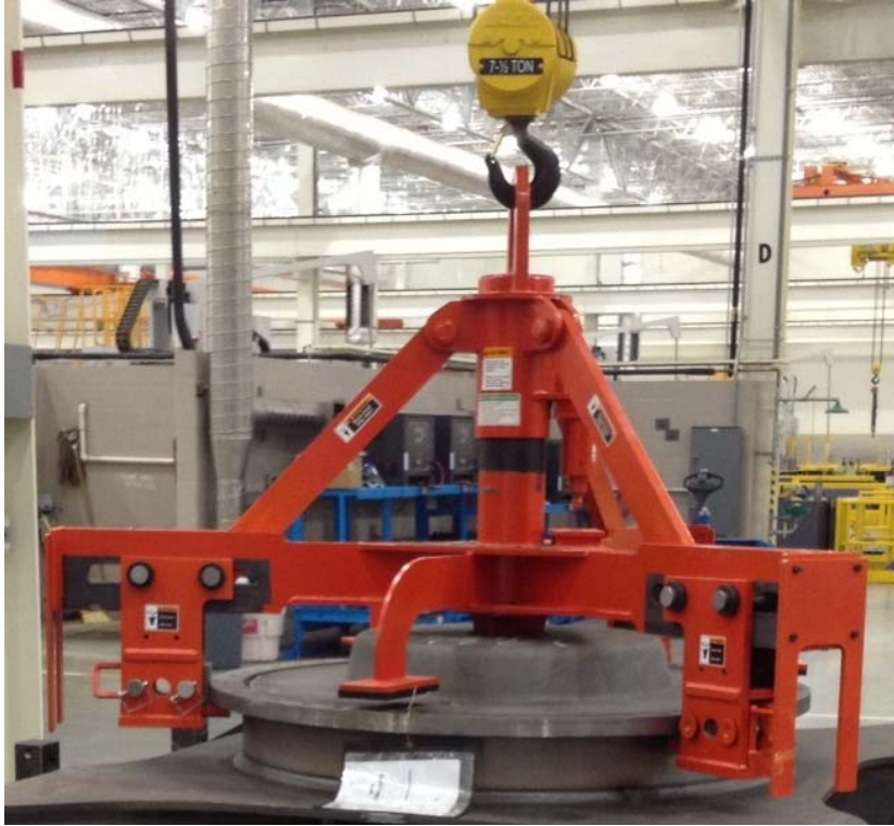
Custom engineered BUSHMAN® lifter picks up one of several sizes of welded frames.
