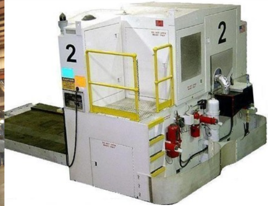
Diesel powered AGV, 35K lbs capacity, hydraulic drive, differential steering, wire guided
