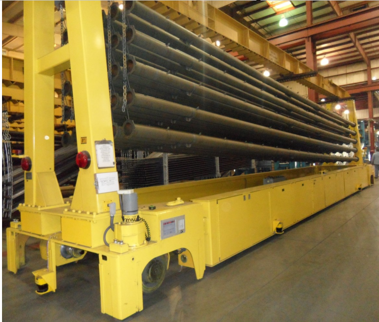
Pipe handling AGV, 51 feet long, 35K lbs capacity, laser guided, 4 drives, 4 steer complete electrical retrofit on site
