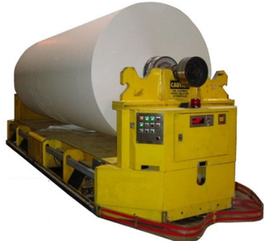
Paper roll AGV 25K lbs capacity, dual drive/steer, wire guided
