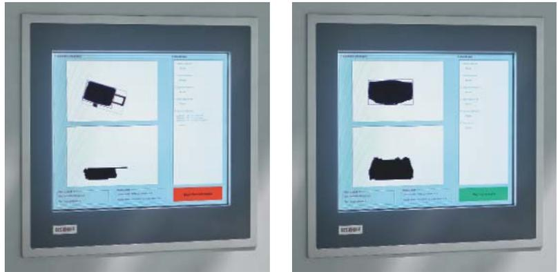
The Control Panel indicates which luggage items can pass through the normal transport route without problem and which items can lead to problems and have to be separated out due to their shapes or special characteristics.
