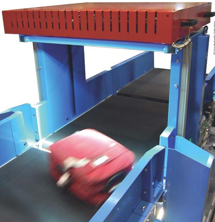
**BAGCHECK in action:** The camera scans 4,000 contours per second when a luggage item passes it (1 contour corresponds to 1 mm). The high exposure and resolution generates a very exact image, based on which problematic luggage items are automatically separated.
