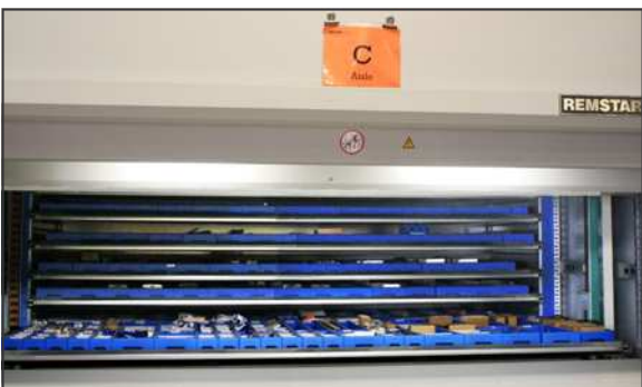
Shuttle has 36 trays storing 1700 part numbers.
