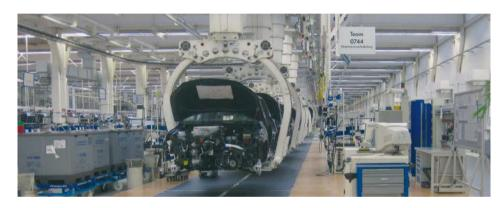
VW in Wolfsburg, Germany, has discovered ultra-flat conveyor denimove as a worker belt. denimove is really flat, and it's exactly that feature that makes it so strong. The motor is integrated into the drive shaft. This is another reason why denimove is so low – in Wolfsburg it's just 12 cm. As the modular belt doesn't slide, but
