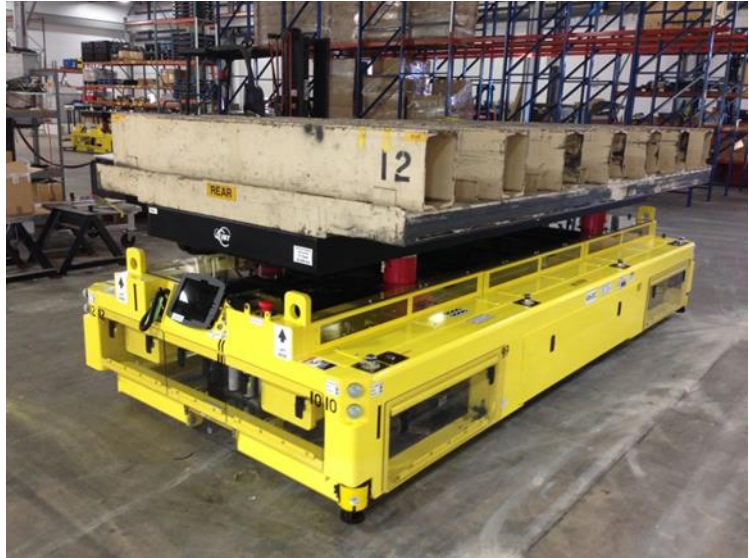
4 Electric Lift Decks and 6 Electric Fork Outriggers work together in a automotive manufacturing plant
