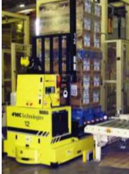
*Laser guided vehicles were installed because of the accuracy and ease with which the paths can be reprogrammed.*
