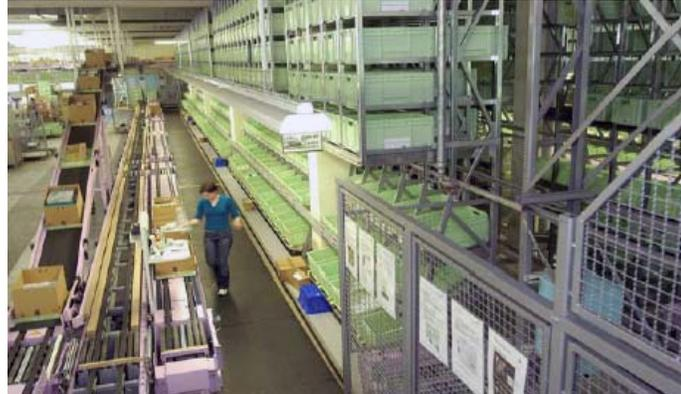
*The High Performance Picking System eliminated replenishment labor and automatically re-slotted slow moving SKU's*
