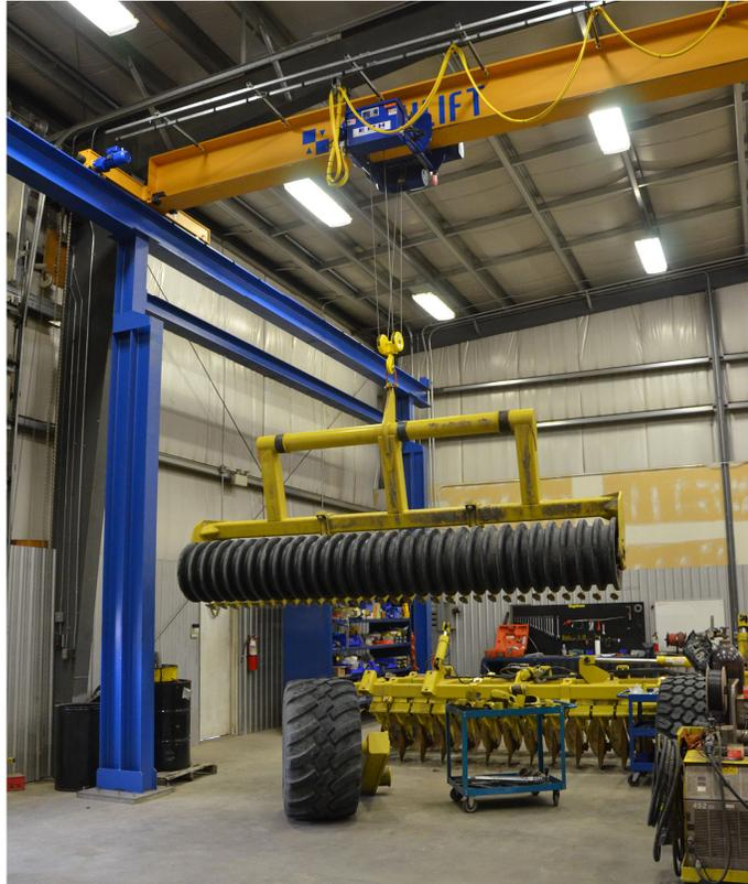
*Acculift, an EMH Distributor, provided Degelman with a custom NOMAD Free-Standing Crane solution.*
