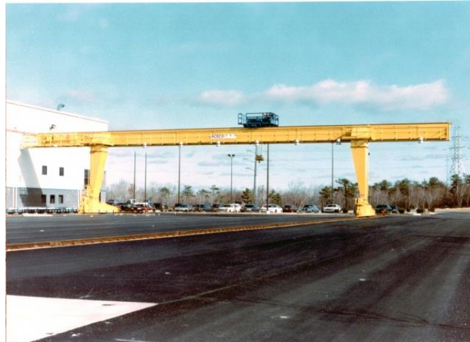
Custom Outdoor Gantry Crane with 150 Ft. Span
