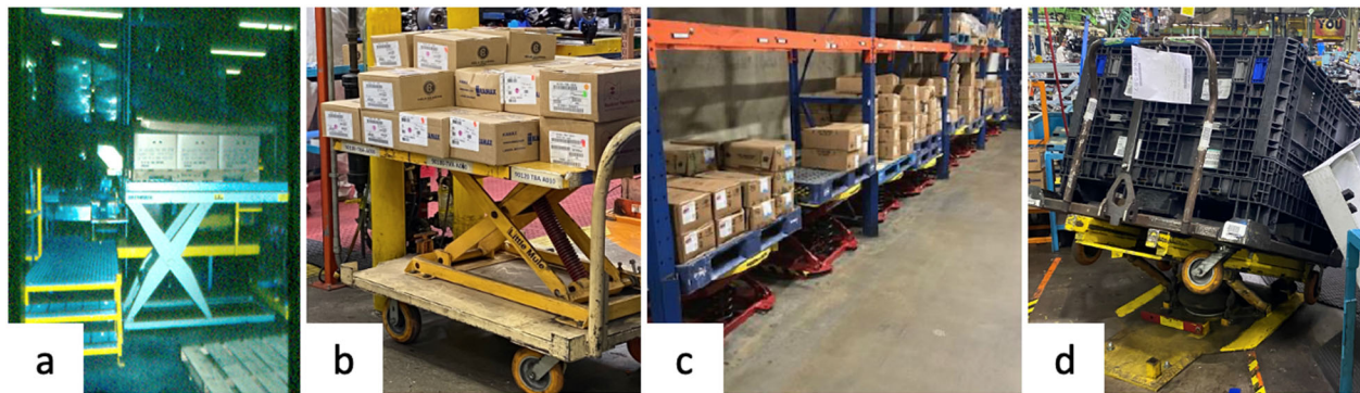
Figure 2. Different types of positioners being used in industrial setting which include (a) a scissors lift, (b) a scissors lift mounted on a cart to facilitate handling and transportation, (c) pallets on self-leveling tables to reduce forward bending in a warehouse, and (d) a tilted bin to facilitate picking.
