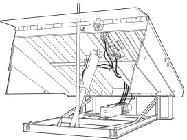
**Hydraulic Pit Leveler** This is the most versatile of the pit style levelers. A hydraulic cylinder is used to raise and to lower the deck, while another is typically used to operate the lip. These levelers may come in various configurations and may be powered by everything from 110V single phase to 575V three-phase.
