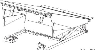
**<u>Air Pit Leveler</u>** This type uses a pneumatic bag system of some type to raise and lower the leveler deck. Obviously, this leveler requires some type of electrical power source - either at the dock or adjacent to it. Most typically, this power source would be standard 110v power. Generally, these levelers are moderately more expensive than mechanical levelers but can involve reduced service and maintenance requirements when compared to mechanical units.
