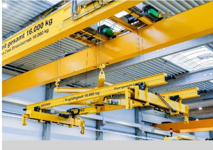
*The SHF 60 wire rope hoists are operated in tandem and are equipped with special articulated trolleys in a particularly low build.*
