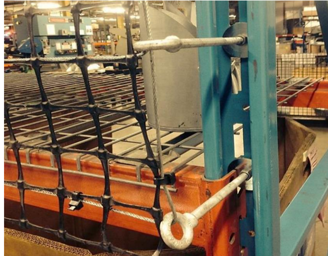
Standard Eye-Bolts Offset Netting from Rack Beams
