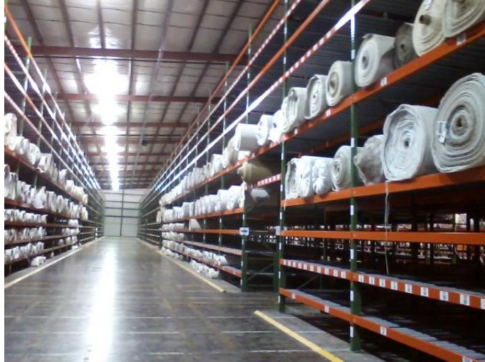
Pallet rack with differentiated shelf spacing and wide aisle optimizes throughput in carpet distribution center.
