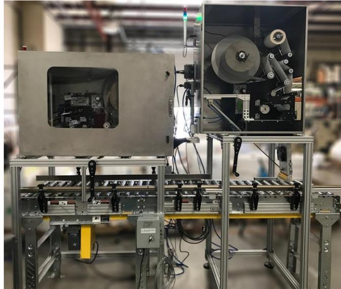
*FOX IV designed a two unit, integrated labeling station to label the various feed block products.*
