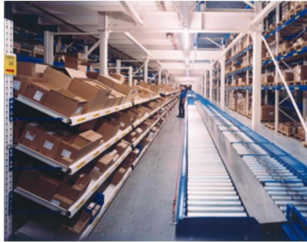
Figure 1: A flow rack representation, flow racks can have very long aisles in a large number of skus configuration.
