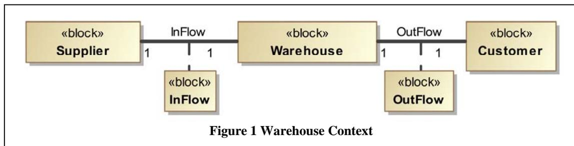
**Axiom 1:** A warehouse has an input flow (InFlow) of shipments from suppliers, and an output flow (OutFlow) of shipments to customers.
