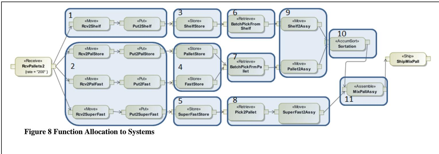
Figure 8 Function Allocation to Systems
