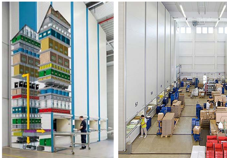
Figure 1. Vertical lift modules
