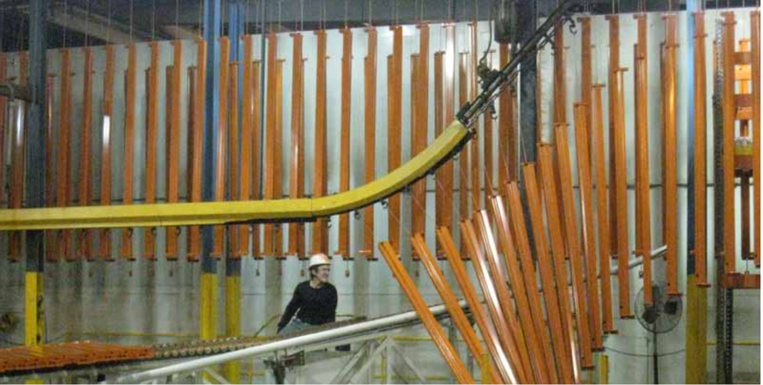
PAINT WASTING TIME, NO MORE: Steel beams sprayed along the line in the powder coating process leave a lot of wasted paint in between each beam. The Interlake Mecalux Plant in South Carolina has continually found ways to minimize such waste.
