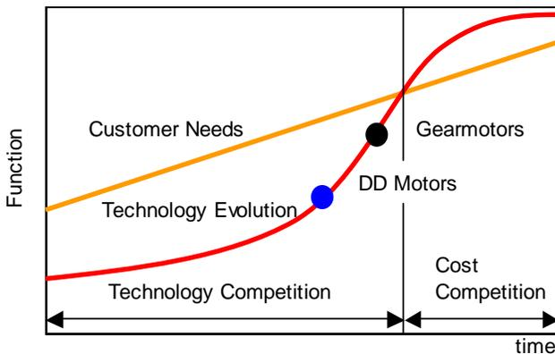
**Fig.12 S-curve of Technology and Customer Needs**
