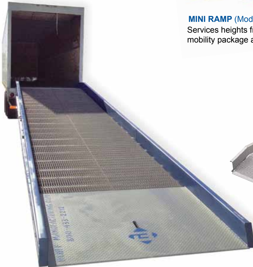
STEEL YARD RAMP (Model YRA) All-welded steel construction with capacities from 16,000 lbs. to 60,000 lbs. Wide range of capacities and sizes available. Double-action hydraulic pump. Solid rubber tires standard, pneumatic tires optional. Available without undercarriage for permanent placement.
