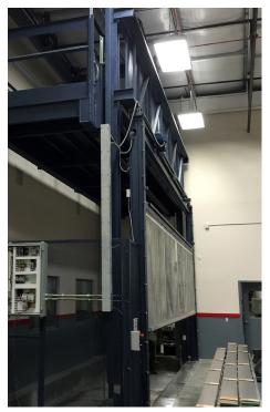
Cardinal Glass is a leading manufacturer of high performance glass for residential windows and doors with 37 manufacturing facilities across the United States. Many of the larger plants feature a PFlow Industries vertical reciprocating conveyor (VRC) to lift components to upper levels during the production process.
