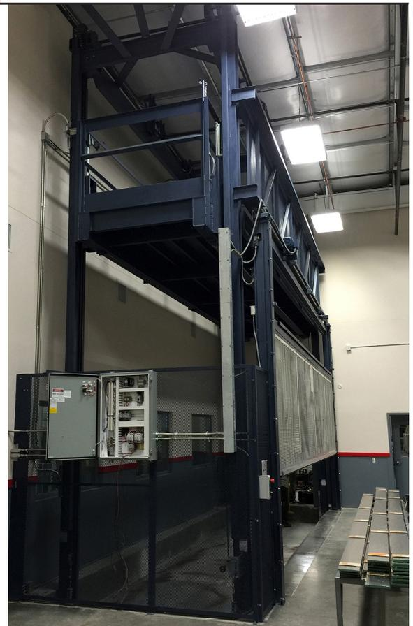
largest engineered and fabricated gates of its kind by PFlow Industries. On the second level, the load exits the lift 90° through an opening with a steel roll-up door; the same narrow opening the forklift had previously used.
