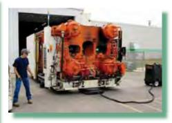
Traksporter allows users more control when moving heavy equipment, by virtue of the fact that it allows a single operator to monitor the various contact points while still able to operate the Crawler via remote control.
