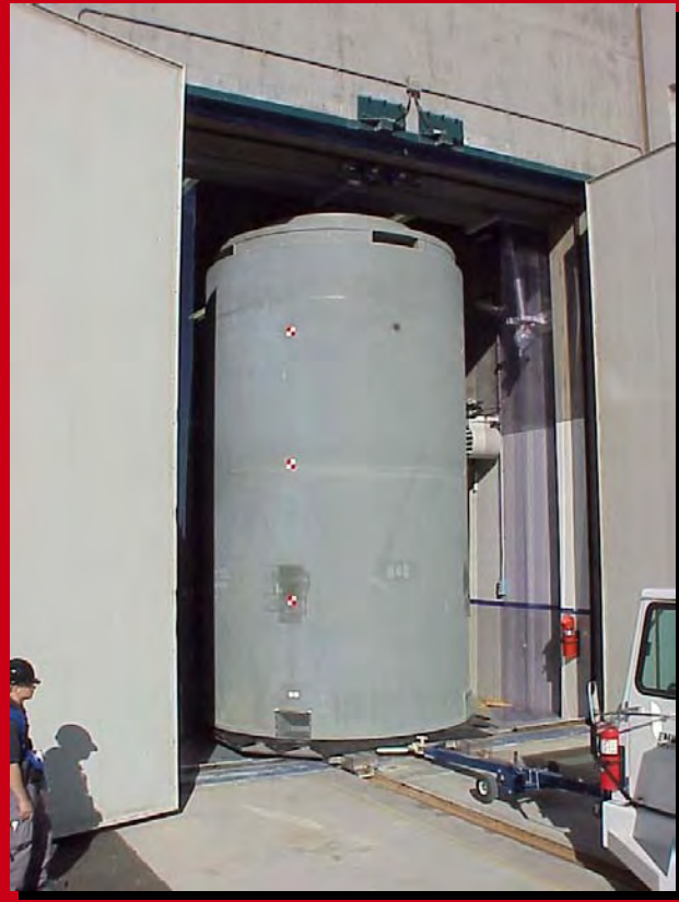
Cask Clears the Door Due to Roller's Low Height
