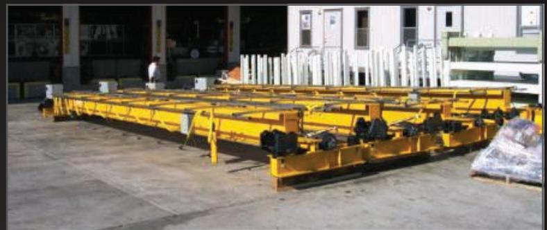
T-Trac bridges ship complete from the factory including all festooning and control components therefore requiring less labor during installation. Ergonomic slim line pendants including all 2-speed buttons with On/OFF come standard on the T-TRAC. The 1HP AC motors complement the drive train of the T-TRAC and are controlled by state of the art variable frequency drives.
