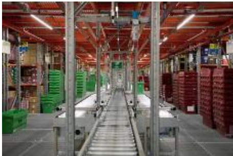
Picture 4: The totes are placed on the roller conveyor and transported automatically to the packing sorter.
