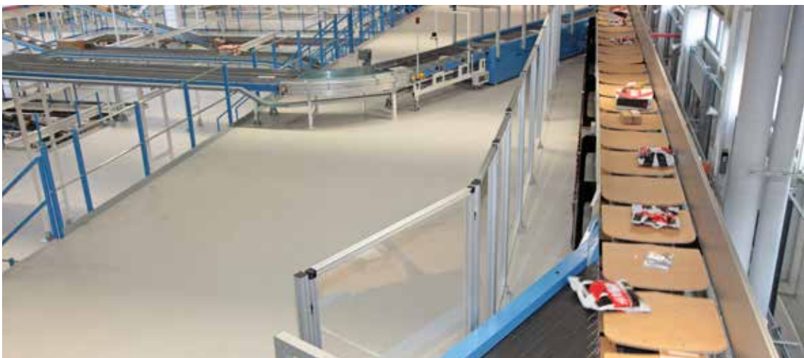
The BEUMER BS-7 Tilt-Tray Sorter is a low cost but durable mechanical tilt-tray sorter perfect for high volume shipping sortation of large retail boxes and small flat poly bags for e-commerce all on the same system.
