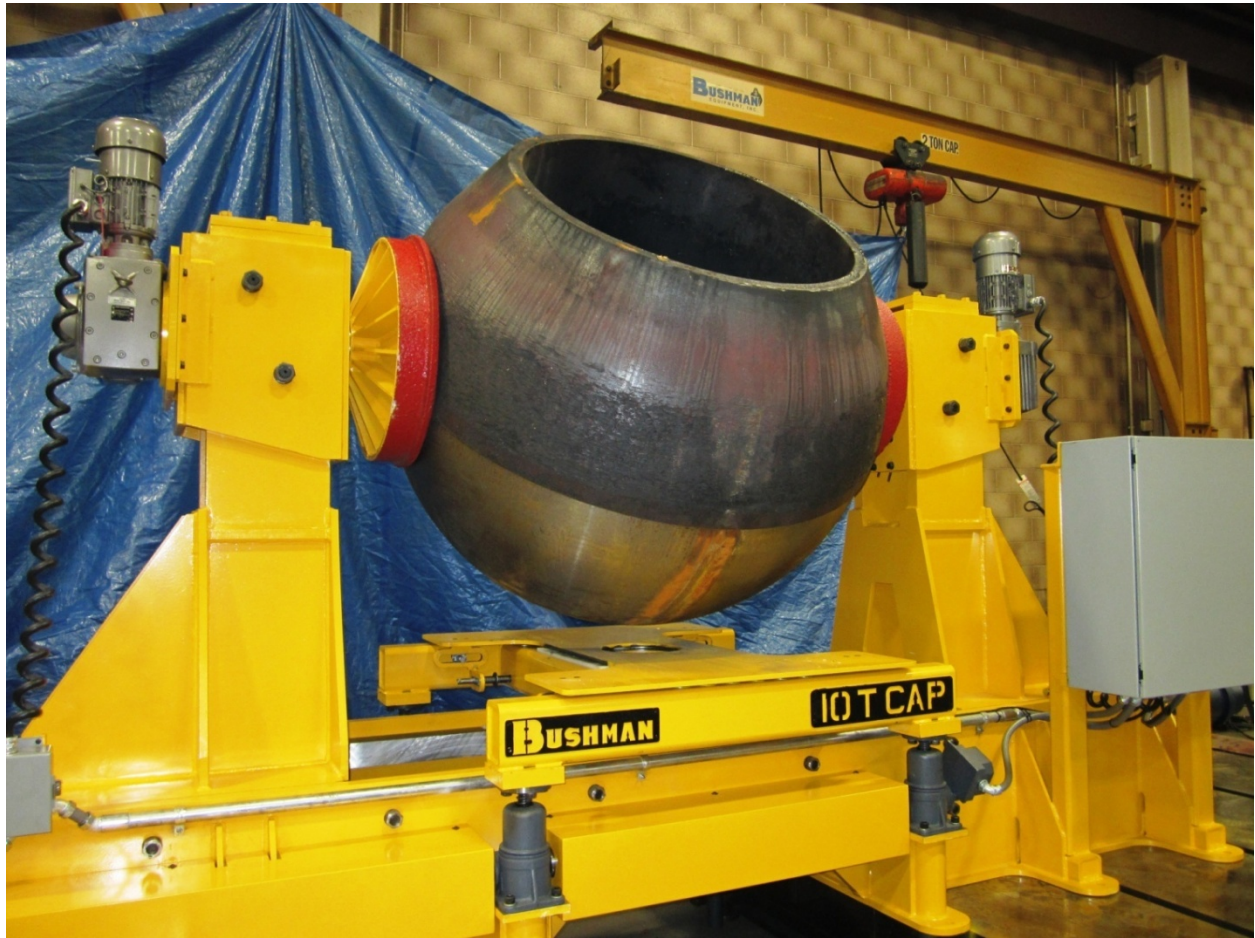
A Bushman Equipment 20,000 lb capacity Clamp-Arm Inverter rotates a steel casting in between machining operations
