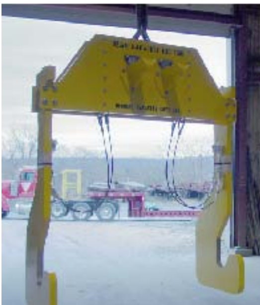
105 ton cask lift beam.
