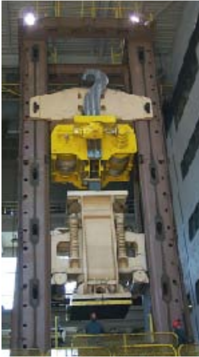
475 ton proof load test of special lifting device.
