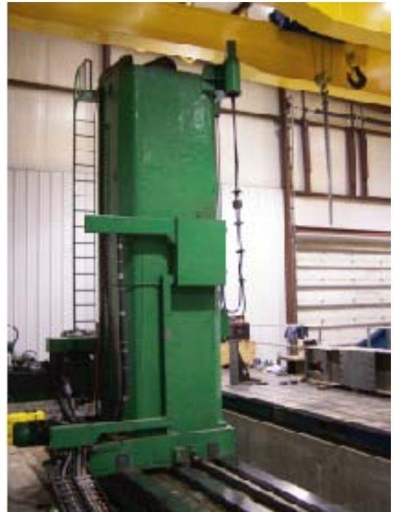
7" Gidding and Lewis floor type horizontal boring mill with 30' horizontal and 13' vertical travel supported with 30 ton overhead crane.
