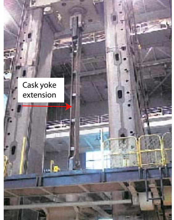
Cask lifting yoke extension shown during 390 ton proof test.
