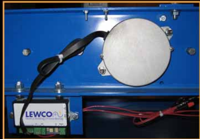
LEWCO 24 Volt DC Motors offer easy to use, plug and play controls
