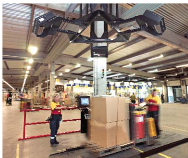
The Cargoscan CSN840 Pallet™ data capture system in action at DHL..
