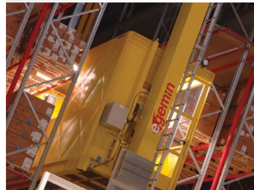
Above: AS/RS pallet crane system
