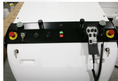
Above: Operator panel with removable manual pendant shown
