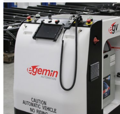
Above: Operator panel with optional touchscreen GDU interface and manual pendant shown
