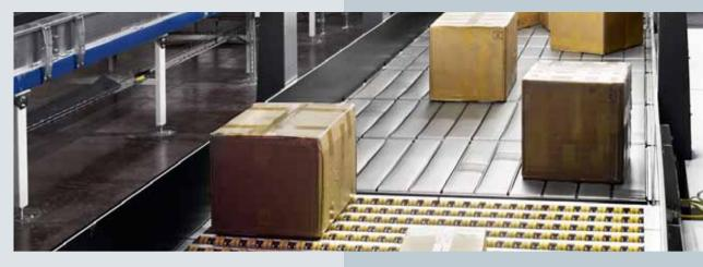
The demand for faster delivery, increased volume and seasonal peaks all impact the throughput of parcel and postal facilities. Singulation of packages in a single pass is an important process required for throughput optimization.
