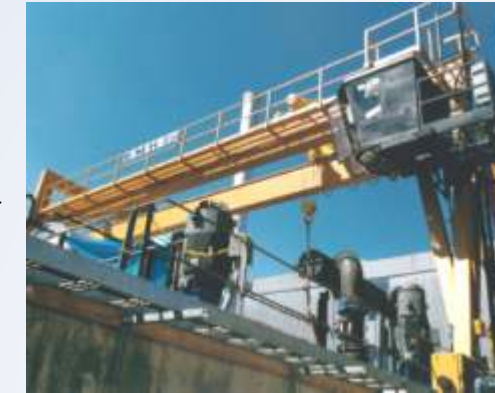
A 25 ton, 120 foot gantry (above) positions architectural concrete panels on trucks for shipment.
