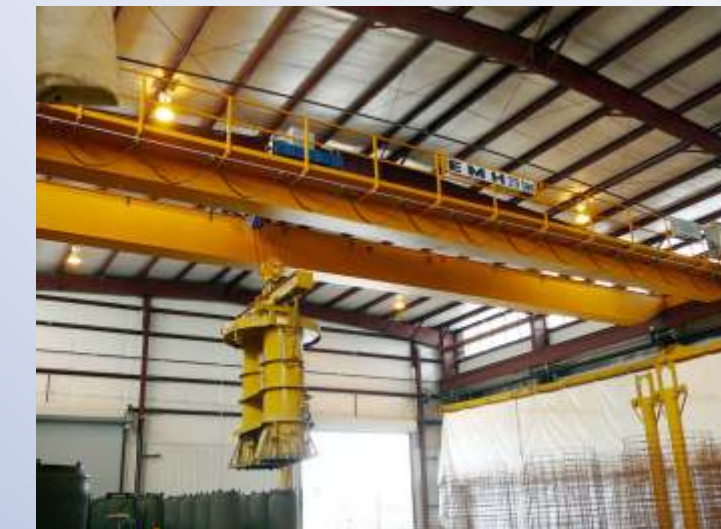
EMH is experienced in building cranes for the concrete industry. The crane at left is used with a Hawkeye machine by a manufacturer of concrete pipe.
