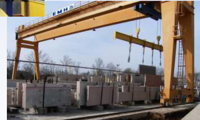
A 25 ton, 120 foot gantry (above) positions architectural concrete panels on trucks for shipment.
