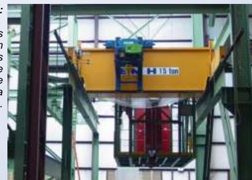
A torsional crane allows high lifts on long spans in a single girder crane. This application uses the crane to set and remove pots of solutions used in a galvanizing operation.
