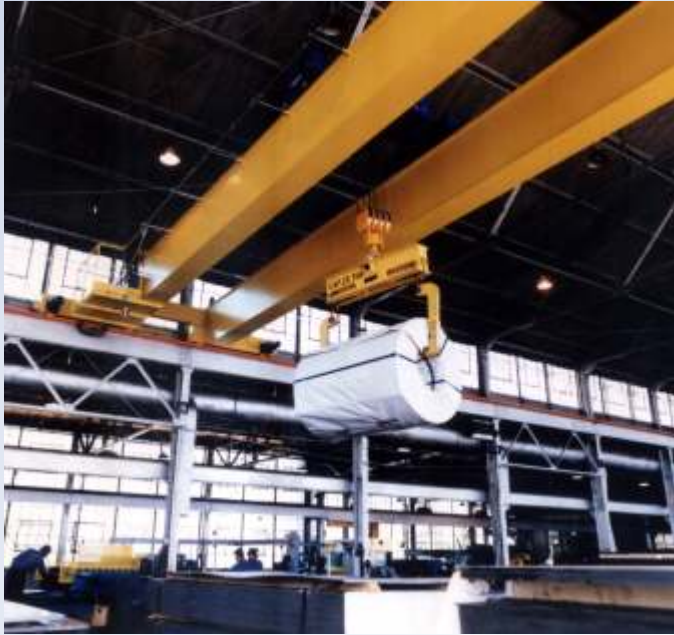
A 20 ton coil handling crane in a steel service center.
