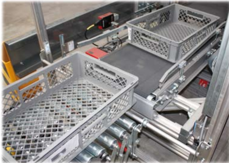
▲ Infeed station of a Portal Lift PH253. Transfer from the roller conveyor to the infeed conveyor. The infeed roller conveyor pivots to separate the trays.
