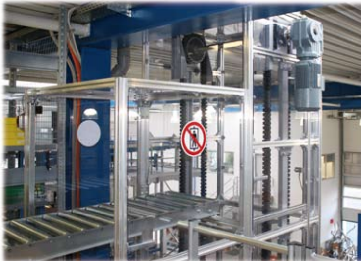
▼ Discharge station of a Portal Lift PH253.
