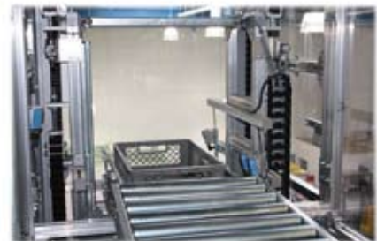
▼ Transfer from a belt conveyor on the lift to the subsequent roller conveyor
